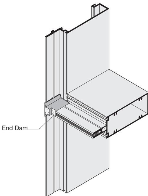
Injection Molded End Dams are sealed in place to control infiltrated water. See page 29-J1 for additional information.
