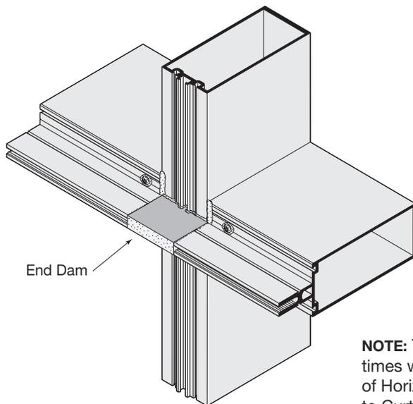
Injection Molded End Dams are sealed in place to control infiltrated water. See page 29-J1 for additional information.
