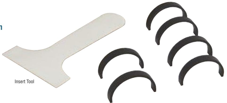
These CRL Anti-Walk Blocks are designed to prevent the glass from "walking" out of the glazing pocket by providing a positive stop in each vertical tube. The coiled rubber blocks can be spread out and inserted into the storefront tube glazing pocket, after which they snap back into their coiled position and stay in place. The AWBT Insert Tool is designed to insert the last Anti-Walk Blocks after the glass has been centered in the opening.
