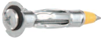
These CRL Drive Fasteners install without drilling. Use a hammer to drive into hollow walls, then a screwdriver to tighten. The tapered tip screw makes driving easy and clean.
