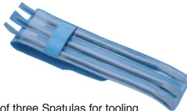
The CRL Sealant Spatula Set is a unique kit of three Spatulas for tooling applied sealants. They are tapered on each end for use in six different joint widths. The lightweight material is strong, will flex under pressure, and is easy to clean up after use. The overall length of each Spatula is 7-1/4" (184 mm), and each set comes in a divided vinyl pouch you can carry in your pocket or toolbox. Minimum order is one set.
