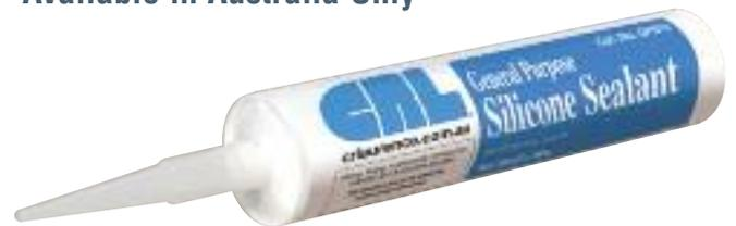
CRL General Purpose Silicone is a one component moisture curing neutral silicone sealant that is easy to use. Designed for general purpose glazing and sealing applications where long term reliability is required, its excellent weathering and UV resistance is important in glazing applications where most organic sealants fail. **SUITABLE FOR:** Zinalume®, Galvabond®, Colorbond®, Marviplate®, glass, aluminium, ceramics, masonry, concrete, stone, most metals, and most painted and plastic surfaces.
