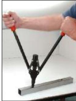
Third, compress the Rivet-Nut by using the CRL Cat. No. 34604 Heavy-Duty Thread Insert Tool
