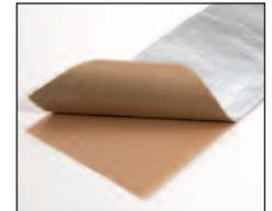
This UL-listed CRL FSK Facing Tape has a 2x3 fiberglass scrim to reinforce it against tearing and stretching. Used primarily as a vapor seal for spandrel insulation panels, it has a special cold weather acrylic adhesive for low temperature performance. It is also used by insulation contractors as a vapor seal for reinforced fiberglass or mineral wool thermal insulation.
