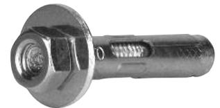
The CRL Red Head Sleeve Anchor is a heavy-duty expansion Sleeve Anchor whose six-rib design assures holding power in cement block, thin wall or solid concrete, brick or stone. Hex nut head allows fastening of numerous fixtures for industrial and commercial applications. Anchor can be installed through objects to be fastened. Maximum work thickness is 1/4" (6 mm).
