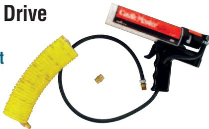
This CRL Deluxe Air Drive Caulking Gun holds all standard size cartridges of sealants, adhesives, mastics or other caulking materials. It weighs less than one pound, so it is easy to handle. The trigger controls material flow, allowing you to dispense a smooth bead 2-3 times faster than a manual gun. It requires 5-70 psi air pressure. The gun comes standard with a 25' (7.6 m) air hose that connects to an optional compressor unit or your own compressed air supply.
