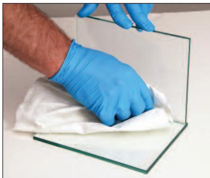
6. Remove Fixtures and Clean Off Excess Adhesive
