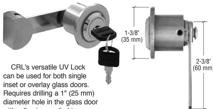
CRL's versatile UV Lock can be used for both single inset or overlay glass doors. Requires drilling a 1" (25 mm) diameter hole in the glass door with adhesive applied to rear surface of cover plate, and bonding the latch to the glass side panel. Each lock includes 1-7/8" (48 mm) short cam for overlay doors and a 2-3/8" (60 mm) long cam for inset door. Each is also designed for 'all-glass' cabinets with a maximum glass thickness of 3/8" (10 mm).
