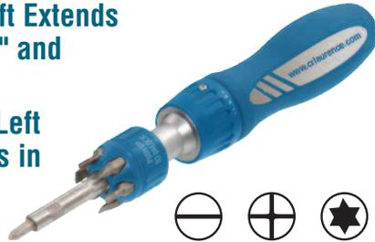
This CRL Ratcheting Extension Screwdriver has a magnetic tipped shaft that extends from 9-1/4" to 15" (235 to 381 mm) overall length. The shaft extends in 1/16" (1.6 mm) increments and locks into place automatically. You retract it by pushing up on the release collar that also holds the six Insert Bits: two each Phillips, Slotted, and Torx. The handle can be made to ratchet left, right, or lock in place. It also features a soft, comfortable grip. Minimum order is one each.
