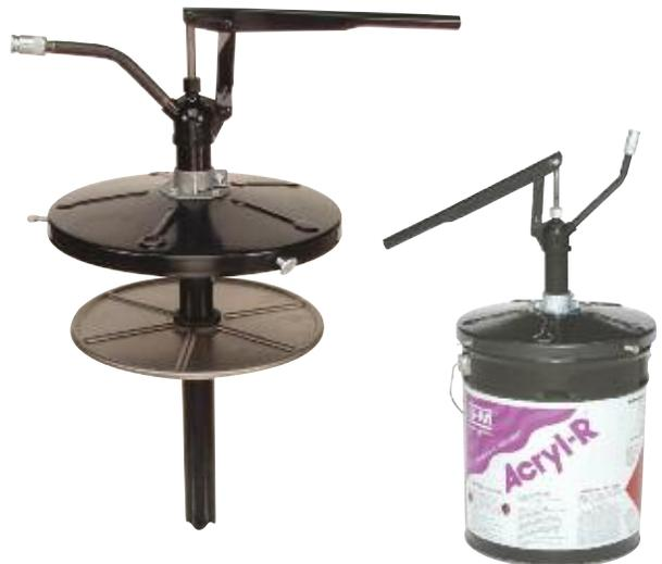
This CRL Gun Fill Pump is designed to transfer bulk sealants, adhesives or lubricants from three or five gallon (11 or 19 liter) pails to convenient smaller containers. It is an 18" (457 mm) pump with 12" (305 ml) cover.
