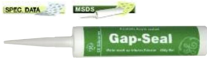
CRL GE® Acrylic Gap-Seal is a flexible, one component acrylic latex caulk for interior and exterior gaps and joints. It displays excellent adhesion to concrete, masonry, wood, brick, glass, ceramic tiles, and plasterboard. It is not designed for joints subjected to significant joint movement or pooling water. Do not apply below 5°C (41°F) or when rain is expected.
