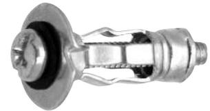
These CRL Hollow Door Fasteners are designed to fasten fixtures where expansion space is too small to accommodate Screw Anchors, such as hollow construction flush doors. Needs only 3/8" (9.5 mm) expansion space. Prongs grip firmly, yet won't split thin materials.
