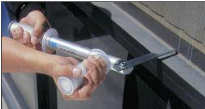
The CRL WT2000 Window De-Glazing Tool is designed for the safe and easy removal of glass lites from their frames. This tool offers you advantages over manual methods because the large handle allows a positive two-hand grip for extra leverage while the heat treated blade cuts through the toughest of sealants. The WT2000 has a three-position handle for easy access to windows at almost any angle or height.
