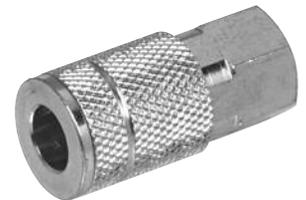
The CRL Female Quick Disconnect Hose Coupler speeds the time it takes to change hoses or tools. Use these brass couplers with the Plug Couplers shown below. Just pull the slide collar back and insert the plug for an airtight seal. Minimum order is one each.
