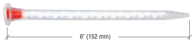
CRL 3M® Auto-Mix™ Mixer Nozzles are the key to 3M® Cat. No. 3M8641 Auto-Mix™ Adhesive. Inside each Nozzle is a series of blades to continually cut and mix the material ensuring that when it reaches the tip it is fully mixed. Each application usually requires a new tip (unless continual flow of material is maintained), so we suggest you stock up on extra Nozzles. Fits Cat. No. 3M8190 3M® Auto-Mix™ Applicator Gun (see page N222). 12 Nozzles per package. Minimum order is one pack.
