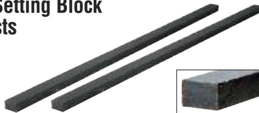
This Windscreen Post Setting Block fits into the glass pocket to support the glass panel at the height you determine. It is made of a rigid UHMW plastic composite that won't compress under the weight of the glass, helping to maintain an even sight line. You can trim it to any length you require.
