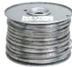
This CRL Strip Lead is ideal for use in making your own custom length setting blocks because the lead is soft and malleable. It will not chip the glass edges, and it can be doubled up for extra thickness if necessary. The 1/2" and 1/4" (12.7 and 6.4 mm) widths come in 1/8" (3.2 mm) thicknesses, in continuous strips wound on 25 pound (11.3 kg) spools.
