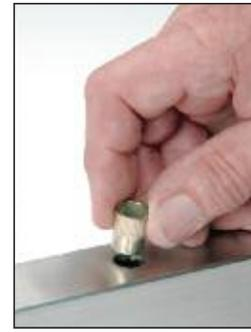
Second, insert the Rivet-Nut into your round post or square tube until the collar on the Rivet-Nut is against the post or tube wall
