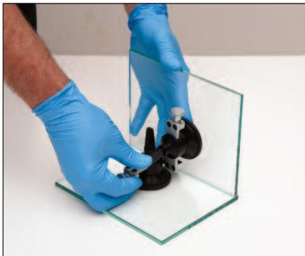
2. Apply Fixtures and Align Joints
