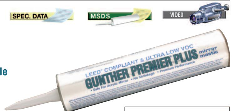
Gunther Premier™ Plus at 72°F (22°C) achieves approximately 30 percent strength in 24 hours, full cure in 7 days. Gunther Premier™ Plus should be applied in 3/8" (9.5 mm) vertical beads, 5 to 6" (127 to 152 mm) apart and away from the edge to prevent squeeze out. Approximate coverage is 7 sq. ft. per cartridge.
