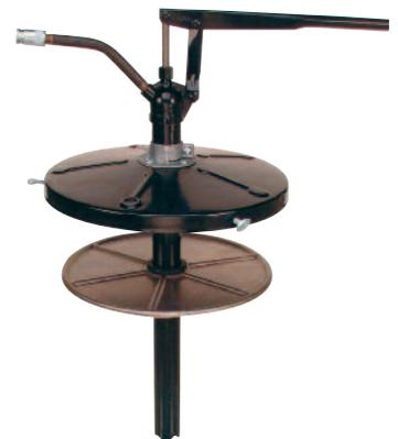
This CRL Gun Fill Pump is designed to transfer bulk sealants, adhesives or lubricants from three or five gallon (11 or 19 l) pails into convenient smaller containers. It is an 18" (457 mm) pump with a 12" (305 mm) follower plate. Minimum order is one each.
