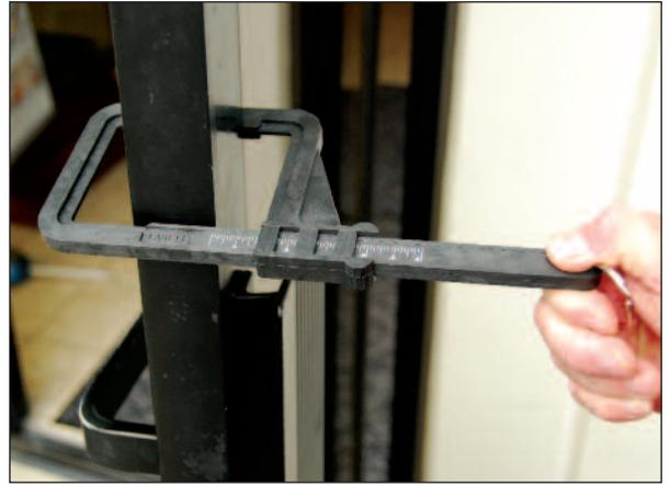
The CRL Insulating Glass Caliper makes it easy to measure the overall thickness of insulated glass panels in sliding windows and doors even when the panels have been glazed into a sash frame. This useful tool will measure up to 4" (102 mm) thick panels. The calibrated scale appears on both sides for quick and convenient measurements. Made of a high impact resistant composite material for durability.
