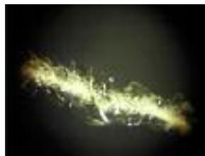
**HEAVY/DEEP SCRATCH** – Above is a magnified image of a heavy/deep scratch. It cannot be removed with this system.
