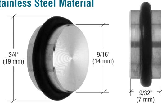
CRL's UV Large Fixed Shelf Support is designed to be bonded to the vertical side panels in 'all-glass' cabinets to support shelving. The Support has a rubber ring surrounding the cylinder which prevents glass movement and scratches. Maximum weight capacity is 44 lbs. (20 kg) each. Minimum order is four each.
