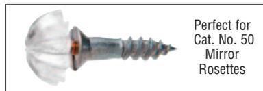
CRL Tapped Head Wood Screws are tapped with a 3-48 machine thread hole to accept CRL Clear Plastic Buds and Threaded Shank Rosettes (online at [crlaurence.com](http://crlaurence.com)). Protect the drilled holes in the mirror by using Vinyl Protective Sleeves (online at [crlaurence.com](http://crlaurence.com)). Screws can be installed with a slotted screwdriver.
