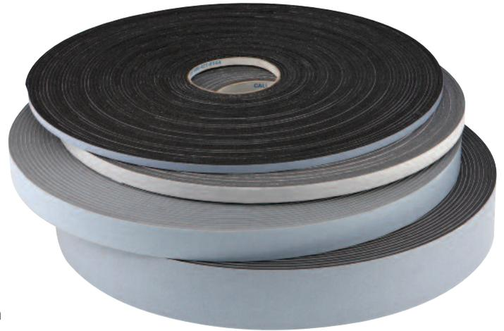
CRL Foam Glazing Tape is a closed-cell polyethylene foam sealant in tape form. The aggressive acrylic adhesive is formulated to position the foam on curved or irregular surfaces with the slightest pressure. Adheres to wood, vinyl, aluminum, and glass. It can be used as an exterior glazing sealant - particularly where glass repositioning is important before the final setting.
