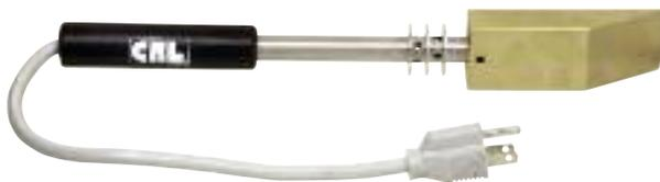
The CRL Insulating Glass Hot Trim Knife trims excess hot melt butyl from single or stacked units. It's the fast and efficient way to finish off single or dual sealed hot melt butyl units. This light, easy to handle Knife can also be used to cut up large slugs of hot melt butyl sealant for faster melting in a thermal extruder system.
