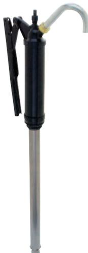
This CRL Barrel Transfer Pump is an easy to operate suction lift pump that can be used on any 30 to 55 gallon (113 to 208 l) drum to dispense a wide variety of liquids. Delivery is 10 fl. oz. (300 ml) per stroke. Features telescoping suction pipe and pipe seal. Excellent for dispensing bulk oil-based sealers or lubricants. **IMPORTANT NOTE:** Not for use with solvents, water-base fluids, weak acids, anti-freeze, or fuel. Minimum order is one each.
