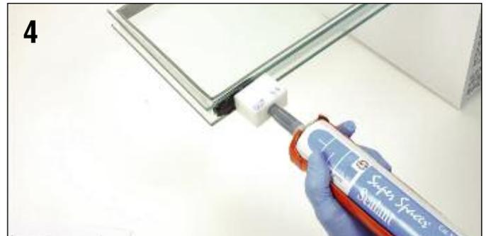
4 Apply CRL Hot Melt Butyl or Cat. No. 877 Super Spacer Sealant to seal the unit
