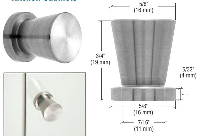
CRL's UV Stainless Steel Knobs are perfect for small cabinets or showcases with glass doors. The tapered knob design is easy to grip and provides a contemporary appearance. The base of the Knob measures 5/8" (16 mm), and extends 3/4" (19 mm) from the door's surface. Minimum order is one each.
