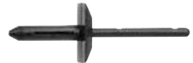
Blind Rivet, Nylon, Door Weatherstrip Retainer; M4 Hole, Panel Range 2.5-5.5 mm, 15 mm x 8 mm Rectangle Head; Saturn '91+
