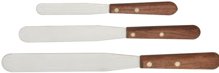
CRL Spatulas are used to tool sealant joints, and to scrape out material from pails. They have a flat, flexible, heat treated stainless steel blade with a rounded tip for creating the recommended hourglass shape of sealant joints. Comfortable hardwood handle.
