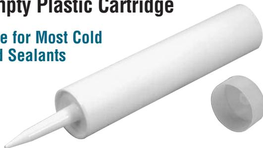
This CRL Plastic Cartridge is made of a high density polyethylene, and is suitable for most cold applied sealants. The 1/10th gallon (310 ml) capacity, 2" (51 mm) diameter, and 8-1/2" (216 mm) length Cartridge fits all standard cartridge caulking guns. The Cartridge includes a tapered, non-removable nozzle and a plunger cap. Minimum order is one each.
