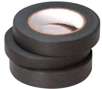
CRL Black Masking Tape is used in between and behind joints of mirror walls to leave a clean black line. This tape also acts as a shock-absorbing cushion when applied to the edge of the mirror, eliminating "clam shell" caused by mirror edges striking each other.
