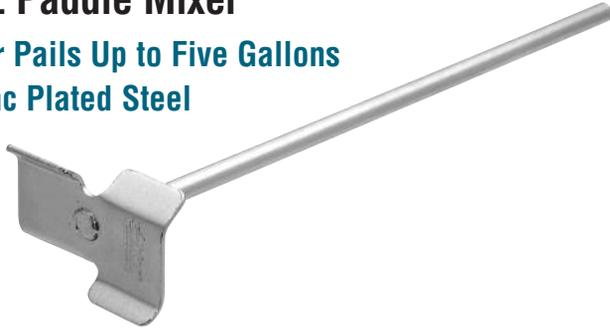
This CRL Paddle Mixer is zinc plated steel and used with larger containers of material, up to 5 gallons (18.9 l). Its opposing bent blades completely mix putties, mastics, paints, sealants, etc. It requires a drill with a 3/8" (9.5 mm) chuck and low RPM. Overall length is 15-3/8" (391 mm). Paddle head is 4-1/4" (108 mm) wide. Minimum order is one each.
