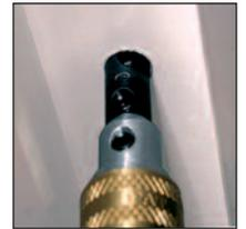
and finishes the hole with the 3/8" Countersink
