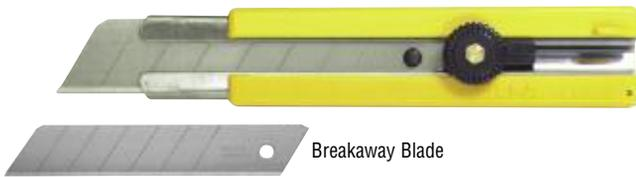
This CRL Olfa® Super Heavy-Duty Knife was designed for the toughest of jobs with a .028" (.7 mm) thick blade that will extend a full 4" (102 mm). A rubber grip handle on the back side provides a non-slip surface for safety and comfort. The H1K uses the heavy-duty 1" (25 mm) wide HB5B Blade shown below. Minimum order is one each.
