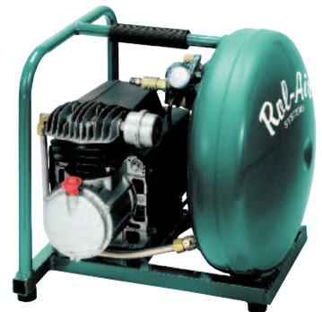
The CRL 2-hp Electric Powered Compressor is sized right for mobile auto glass trucks and vans. It comes with a 2-hp 3,400 RPM electric motor that features overload protection with manual reset. This Compressor is a single stage, ball bearing design to provide years of reliable service. The Compressor's footprint is only 16" x 16" x 16" (406 x 406 x 406 mm). Minimum order is one each.
