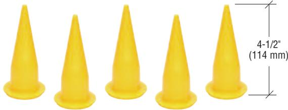
CRL Yellow Plastic Cone Nozzles are extra large for bulk and sausage caulking applications where wide beads of material are required. These are the same Cone Nozzles that come with the Cat. No. WG51001 Sausage Gun. The plastic cone-type Nozzle can be cut to deliver a bead from 1/8" to 1-5/16" (3 to 33 mm) in diameter. Fits most sausage and bulk guns with screw-on ring caps. Five Nozzles per pack. Minimum order is one pack.
