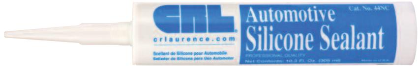
CRL 44NC Neutral Cure Automotive Silicone Sealant is a fast curing, neutral cure silicone with special adhesion additives for use in vehicles to seal and weatherproof. It stops leaks while cushioning the glass against shock and vibration. Easy to dispense, this one-part formula features primerless adhesion to aluminum, stainless steel, chromium, tin, iron, plastics, silicone gaskets, rigid PVC, phenolic resin, glass, ceramic, and most reflective-coated glasses.
