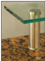
CRL UV Pole Supports can be used to support a flat glass shelf, bar, or table top at 5-1/2" (140 mm) above the bottom surface. Fabricated from stainless steel for strength and corrosion resistance, these vertical Supports can be installed into wood bases by drilling a 7/16" (11 mm) hole, or into granite or stone by drilling 5/8" (16 mm) diameter holes. Minimum order is one each. **CAT. NO. UVCD30**
