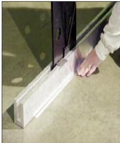
CRL Aluminum Shim Strips are used under one side of Heavy Aluminum Base Shoe to adjust it into a plumb position before securing it with the fasteners. The length can be trimmed as required for an exact fit.
