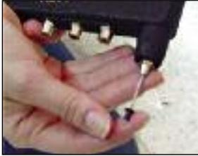
1. Insert rivet mandrel in rivet setting tool.
