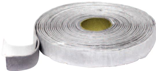
Use CRL Putty Tape to seal between the vehicle body and frames of aluminum windows. Originally designed for manufacturers of mobile homes, campers and RVs, the material stays soft and pliable, so it installs easily and conforms well to corners. It comes rolled on specially treated release paper for easy handling, and is easy to clean up.
