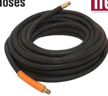
The CRL 3/8" (9.5 mm) diameter Premium Air Hose is made from genuine Goodyear Rubber with 1/4" (6.4 mm) male NPT brass fittings on both ends. One end has a special kink resistant sleeve. Rated for pressures up to 250 psi (17 bars).
