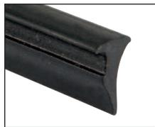
This CRL Tremco® Wedge Gasket Glazing Spline profile is made of extruded 70 durometer dense EPDM. The wedge profile is designed for use in compression glazing systems with Tremco® POLYshim™ II Glazing Tapes. Glazing Spline profiles require a .090" x .062" (2.3 x 1.6 mm) metal nib for proper engagement. **NOTE:** A mock-up is recommended by Tremco® to verify acceptable mating between both the Glazing Spline and the metal nib.
