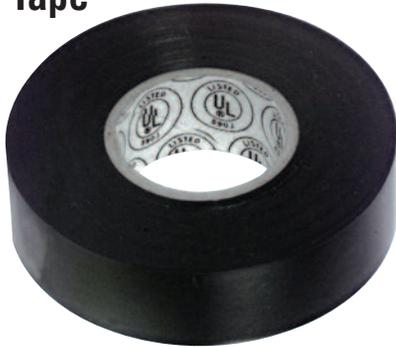
Designed to insulate wire, pipes, dissimilar metals, etc., CRL Electrical Tape is resistant to weather, water, acids, alkalis, and oils. It has superior conformability and high elongation to give a tight, solid wrap. A silicone spray additive gives it an 18-month shelf life. It practically never telescopes or bleeds. The glossy black tape is 7 mils (.18 mm) thick.
