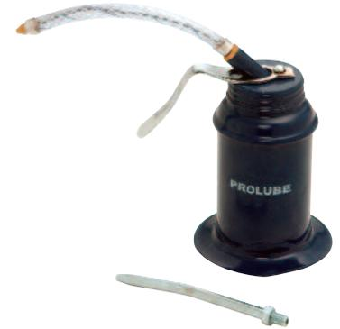
This heavy-duty CRL Pistol Type Oiler dispenses oil and solvents through either a 6" (152 mm) rigid metal, or flexible high density polyethylene spout. It has a 6 fl. oz. (177 ml) capacity and supporting base ring. This oiler also features a brass pump mechanism for smooth operation and a gasket on the lift rod to prevent leakage. Baked-on enamel finish on the body resists rust.
