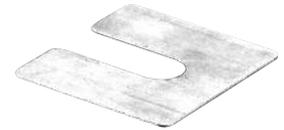
Aluminum Horseshoe Shims are available in three thicknesses for use with SurfaceMate Base Shoe. Shims are slotted to allow for minor adjustment, and can be stacked in various sizes to accommodate irregular surfaces below the base shoe and curved block. They can also be used in fascia mount applications of SurfaceMate Base Shoe.
