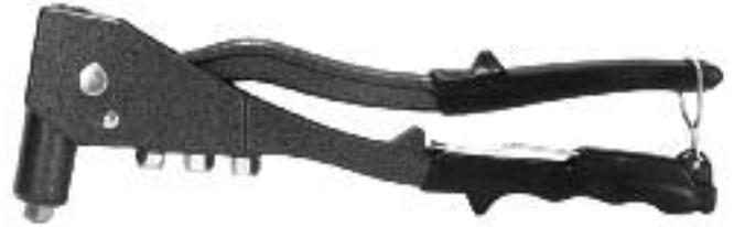
This CRL Manual Rivet Gun is smooth and fast. Interchangeable nosepieces attach to the base when not in use and will set 3/32", 1/8", 5/32" and 3/16" (2.4, 3.2, 4, and 4.8 mm) rivet sizes. Minimum order is one each.
