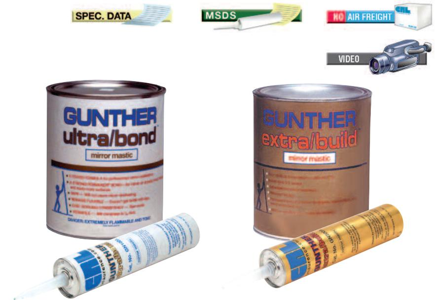
Gunther Ultra/Bond's viscosity provides for a build out of 3/4" (19 mm), and can be compressed to 1/32" (.8 mm) for mirror installations requiring close tolerances, such as overlays, mirrored furniture, and medicine cabinets. At 72°F (22°C) it achieves approximately 30% strength in 24 hours, full cure up to 605 psi in 30 days. It comes in 10.1 Fl. Oz. cartridges and one gallon cans.
