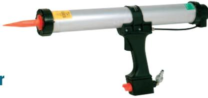
The CRL Cox Air Power Sausage Caulking Gun dispenses even heavy materials, such as urethane, at a smooth, controlled rate of flow. It can be used with 10, 15.2 or 20.3 fl. oz. (296, 450 or 600 ml) sausage packs. The high flow trigger valve is responsive, with a built-in regulator to control flow, and an instant release valve with silencer to stop material flow. Can operate at up to 100 psi maximum. Minimum order is one each.
