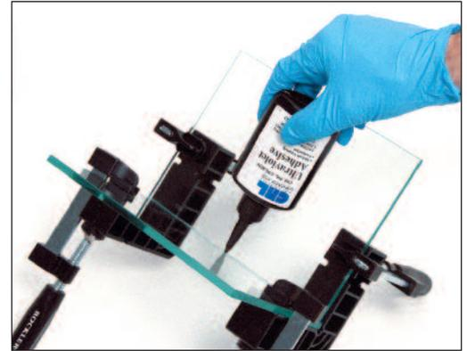
An important fact to always remember is that the smoother the bonding surface and the thinner the layer of adhesive, the stronger and more resilient the bond will be. A layer of too much adhesive reduces the strength of the bond, and increases the workload of removing excess adhesive.
